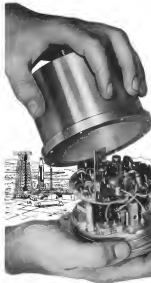
Donner's rugged new angular accelerometer weighs only 2 pounds
